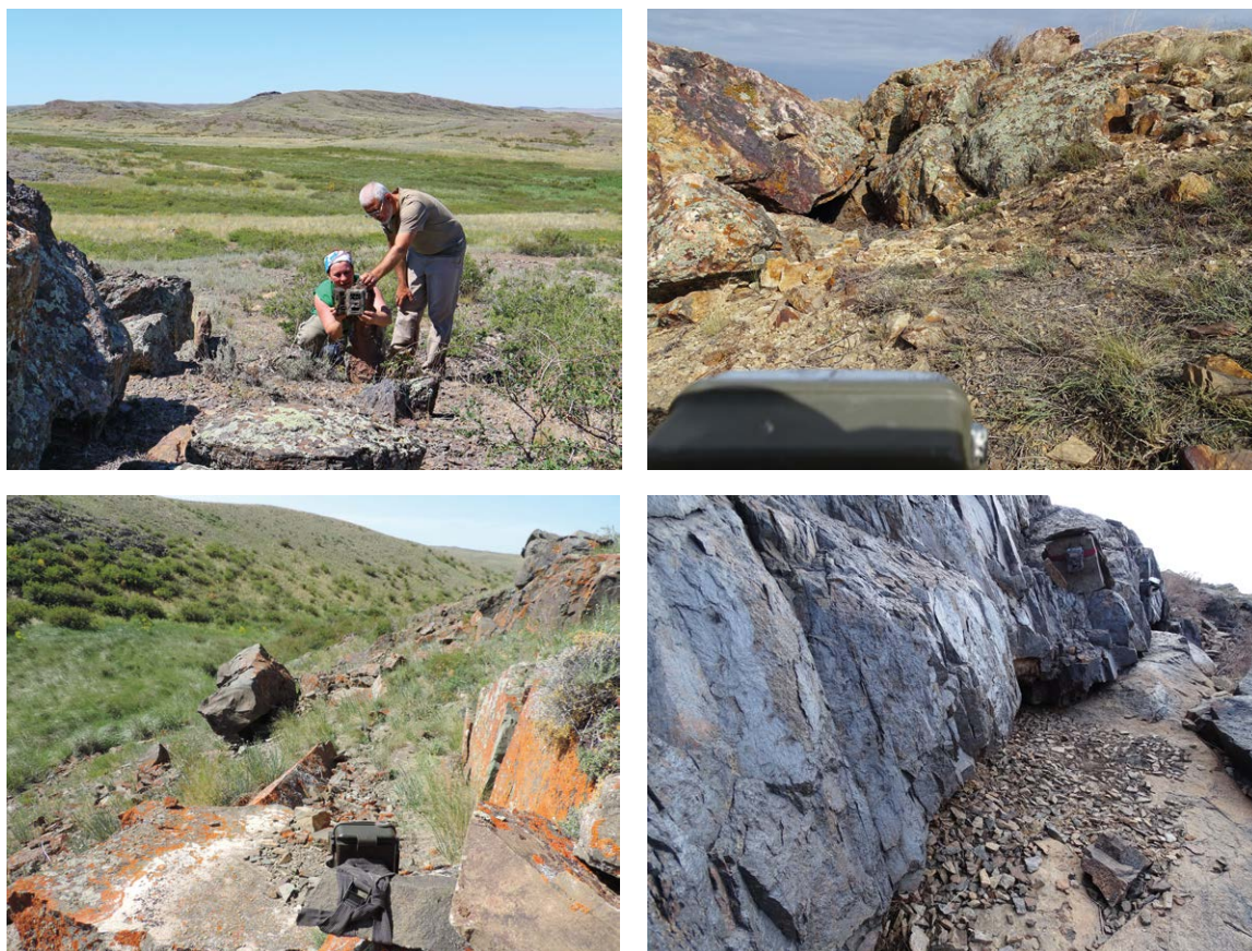
Figure 23: Before leaving the camera station, make sure to check that the camera is placed at the right distance and angle from the focal area and that the camera's viewshed is not obstructed. Placing the camera almost parallel to the focal trail is the best option in most situations for maximising manul detections. However, in some locations the camera needs to be oriented on an angle of less than 45° relative to the focal point for better results. Photos: A. Antonevich, I. Smelansky, A. Barashkova
