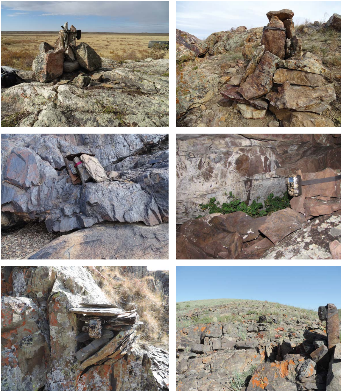
Figure 9: Elements from the environment can be used to set up a camera station at the height and angle of interest. Rust-resistant, heavy duty mounting straps and cable locks are useful to tighten up the camera around a rock, tree, or pole. However, these attachments may loosen over time and should be monitored during long-term studies. Photos: I. Smelansky and A. Barashkova
