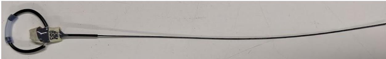
Figure 1, the constructed transmitter belt with silicon tubing, PVC tubing and catgut.
