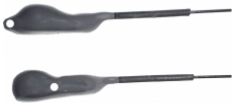
Figure 10, two designs of a BD-2 transmitter of Holohil Systems Ltd., One with a frontal anterior tube (top) and one with a center tube (bottom) (17).
